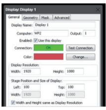
Note: If you want to use WATCHPAX without a display, e.g., as a sound server, set a "dummy" resolution of 640x480 pixels in WATCHOUT. In that case you need to use an <u>active</u> MiniDisplayPort adapter to DVI/VGA/HDMI to ensure that the correct EDID infomation is transferred to WATCHPAX.
